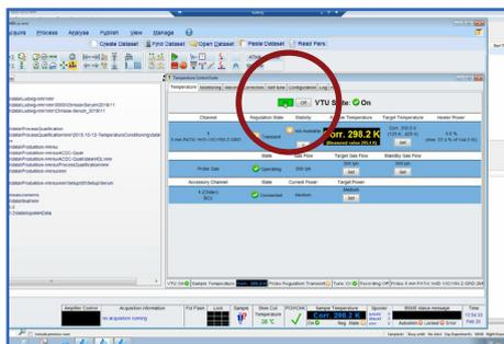
Open the TopSpin Software and switch on the vtu temperature control. Wait until temperature display is green.
