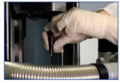
Remove the old pincer by slowly turning while simultaneously pulling it off.
