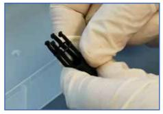
Make sure that the o-ring is placed in the second indentation of the pincer's sleeves.
