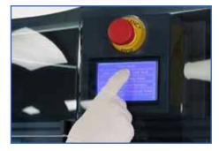
To access the gripper arm in the SampleJet, push "Load rack" and select any rack number of options 1 through 5 on the SampleJet Touch Display.
