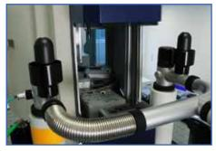
To access the gripper arm, ensure the cover of the SampleJet is pushed upwards.
