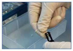
Prepare a new pincer by pulling the o-ring over the pincer's sleeves.
